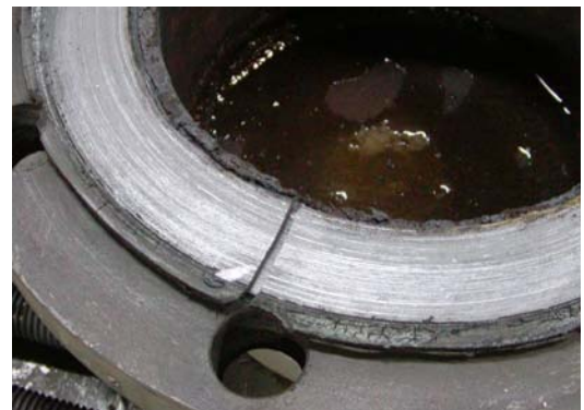
Figure 10 - Blow-out failure of Style A
