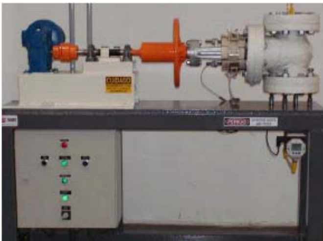
FIGURE 9 – GATE VALVE TEST BENCH
