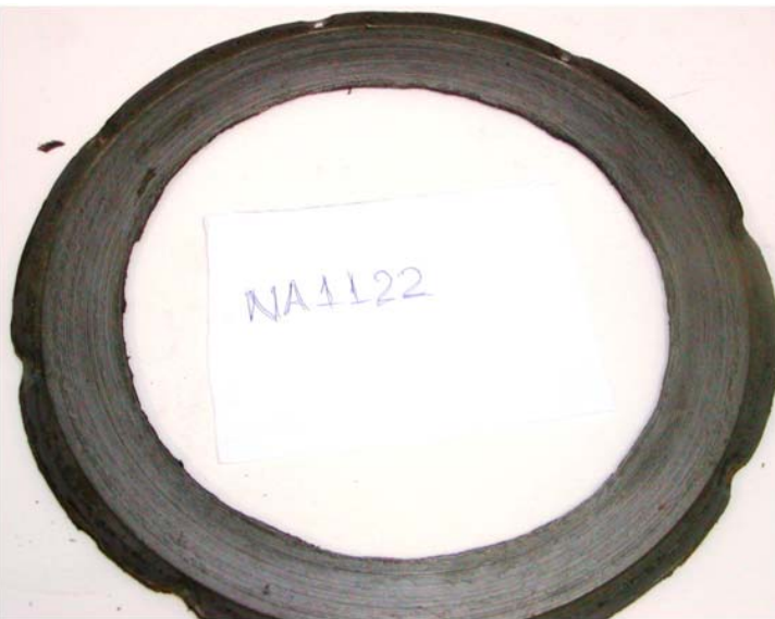
Figure 6: Teadit NA1122 after disassembled.
