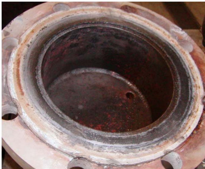
Figure 4: Teadit NA1122 after test.
