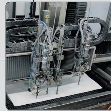
Computer Controlled Gasket Cutting
