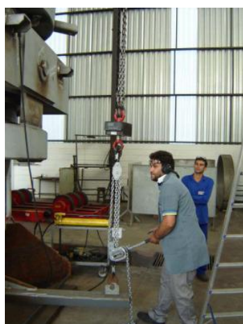
Fig. 5. Test Device. (a) Dynamometer used during the test, (b) angle measurement device and (c) Load application.
