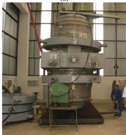
Fig. 4. Expansion joint in the test position (unit in mm). (a) Schematic draw of the test device and (b) Test device build of.
