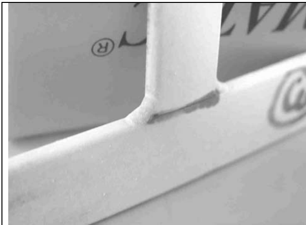
Figure 4 – Penetrant test after compression
