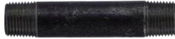
1/2" DIAMETER BLACK EXTRA HEAVY XXS SEAMLESS Wall Thickness 0.294 - Grade B - Test Pressure 1000 PSI - Thread Length 0.79
