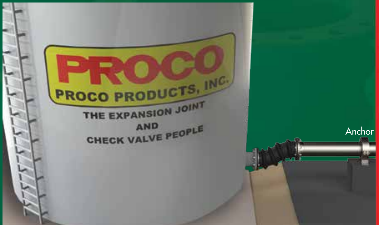
Tank After Settlement
