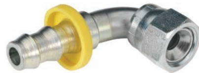
Female Swivel 90° Elbow 37° JIC/45° SAE-Plated Steel
